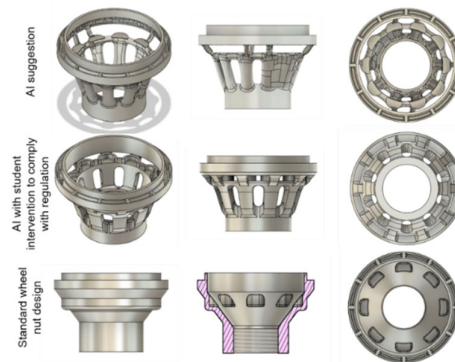
Figure 4. Generative design shape optimisation (top - Fusion360 generative design, middle – modified by student to comply with regulation, bottom – standard wheel nut design)
