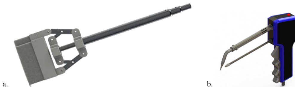
Figure 4. Idea generation based on trend of (a) increasing controllability – a flexible broom, and (b) increasing completeness of system component – an automatic feeding solder
