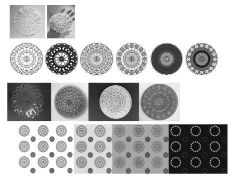
Figure 3: 1st line top: Original lace in cotton - handmade by the grandmother of one of the authors (Lyche). 2nd line: Original lace drawn in illustrator, 3rd line from left to right: A: Simplied lace cut in Dycem lasercut. B: 3D print mould of lace- used to make silicon sample. C: Liquid 3D print mould of lace- used to make silicon sample. D: Silicon sample from liquid 3D mould. Bottom line: Surface pattern design made from original lace with different colour settings. All designs by Lyche
