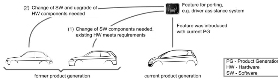
Figure 6: Transfer of features to former product generations and necessary
