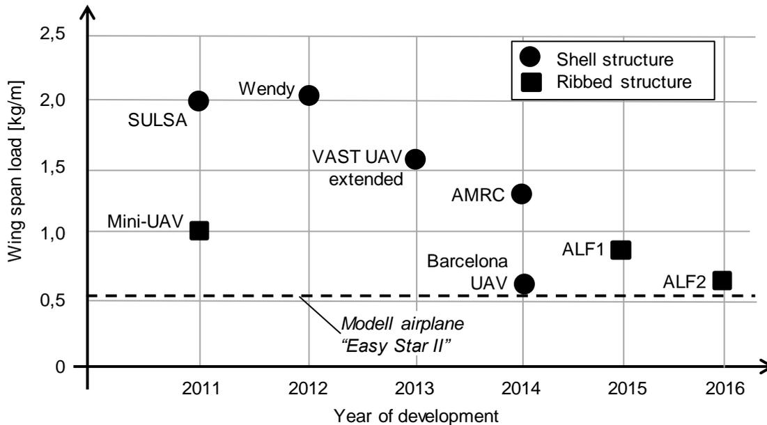
Figure 7: Comparison of the wingspan load for various 3D-printed UAVs with model airplanes made of foam (adapted from Junk and Schröder, 2016)
