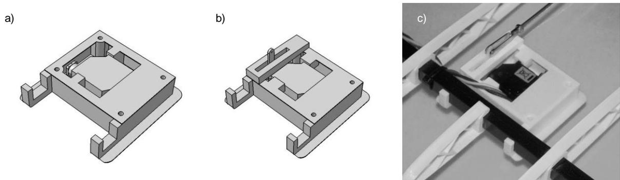
Figure 5. Design of servo bracket before (a), after passing through the main development cycle (b) and as 3D-printed (FDM) and mounted component (c)
