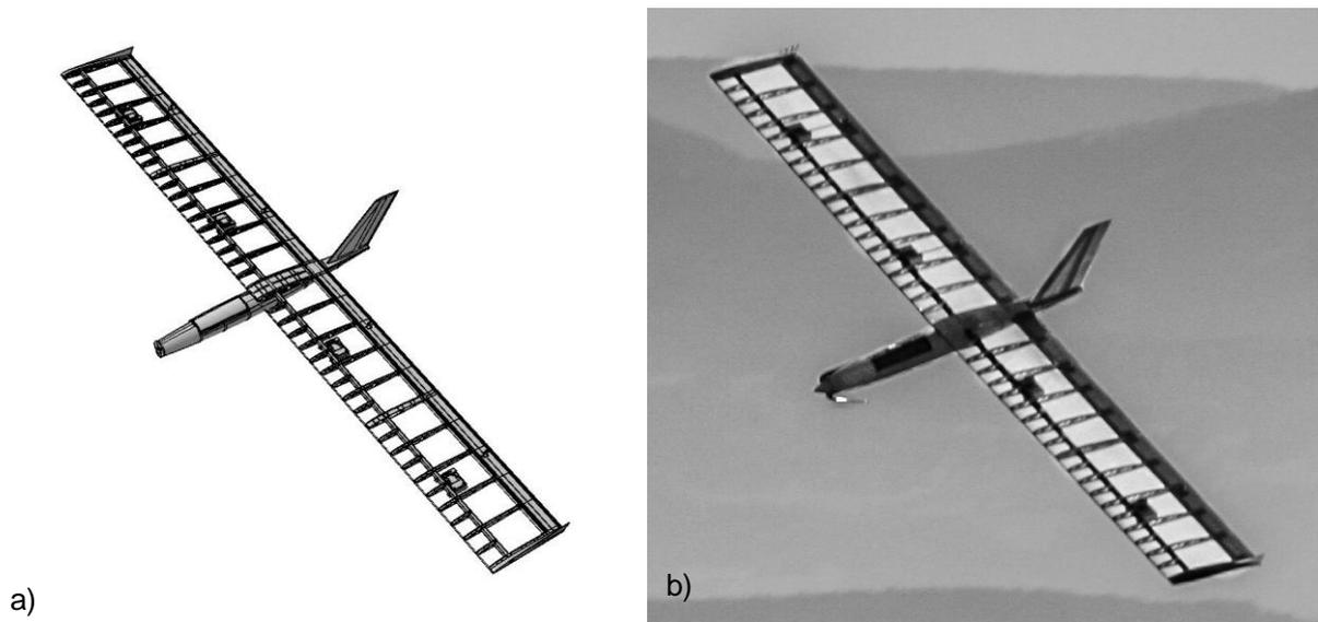
Figure 2. UAV named ALF 2: CAD model (a) and UAV during flight test (b)
