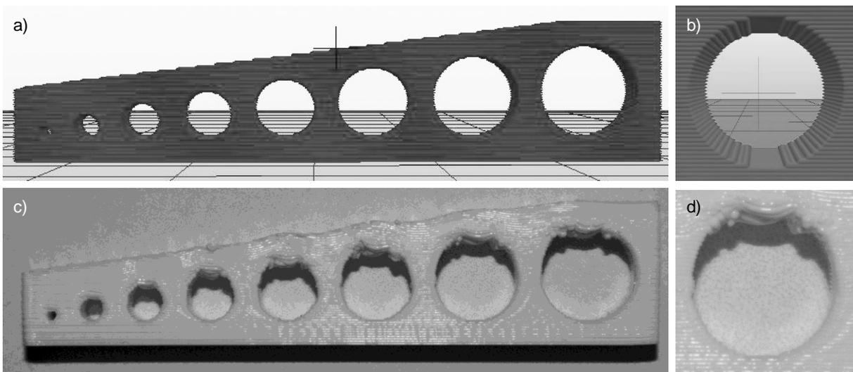
Figure 4. Determination of the process limit for the production of holes without support structure in Pre-processing (a) with detail of the gradation of the individual layers (b) and as test component using FDM (c) with detail of incidence in the upper region of the hole (d)
