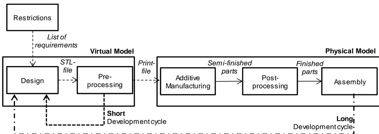
Figure 1. Development cycles in Design for Additive Manufacturing (adapted from Junk and Schröder, 2016)
