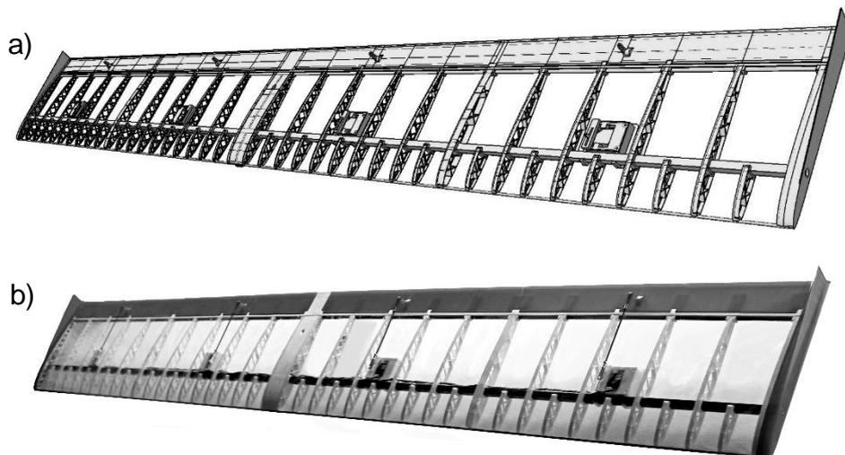
Figure 6. Design of the wing in the CAD software (a) and mounted wing with components from 3D printing using FDM (b)
