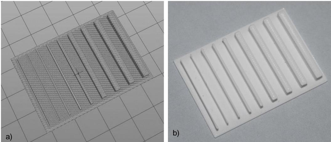
Figure 3: Determination of the process limit minimum wall thickness in Pre-processing (a) and as 3D printed test component using FDM (b)
