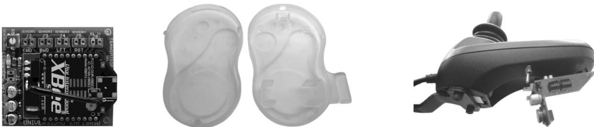
Figure 11. (a) Transmitter PCB (b) Earphone case (c) Receiver PCB on wheelchair
