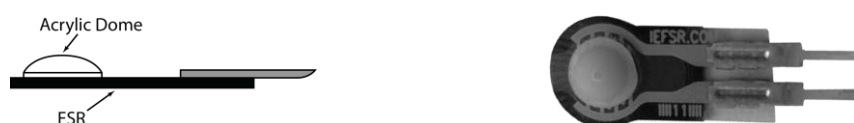
Figure 5. (a) Side View of FSR with acrylic dome (b) Upper View of FSR with acrylic dome
