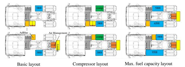
Figure 6. Exemplary layouts produced by the presented methodology (bottom row) compared to original layouts of the current product generation (top row)
