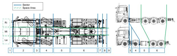
Figure 2. Generic package space decomposition at MAN. Highlighted sectors 3, 5 and 7 show possible installation space for chassis mounted parts.
