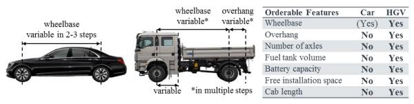
Figure 1. Differences between car and truck
