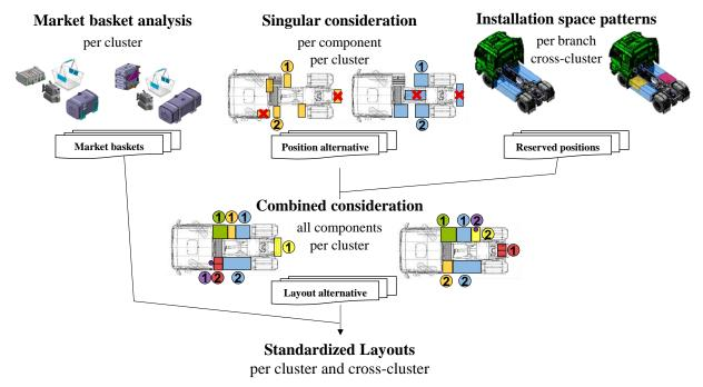
Figure 3. Methodology for deriving standardized layouts
