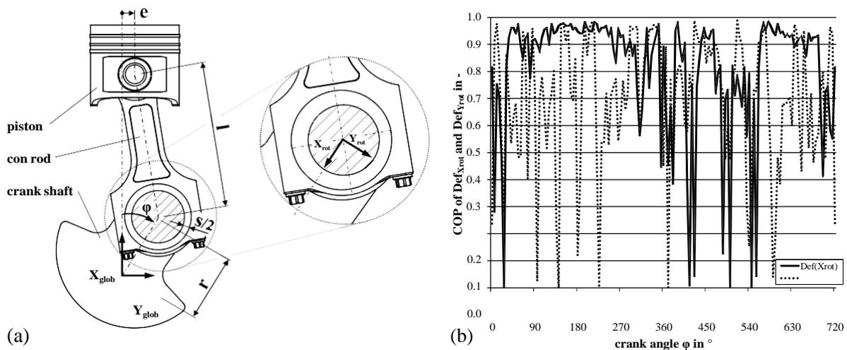
Figure 2 (a) Crank mechanism (b) Time-dependent COPs of the crank deformation
