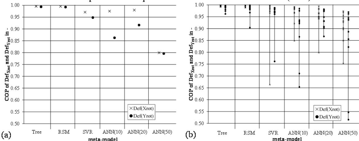
Figure 3 COPs of meta-modeling techniques: Split- (a) and Cross-Validation (b)
