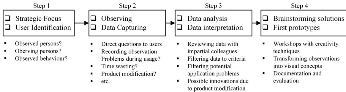
Figure 2. Process of empathic design based on (Lüthje, 2007) and (Morris & Cormican, 2012)
