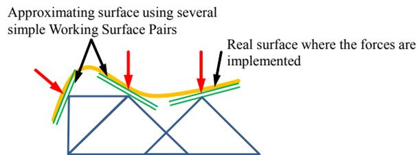
Figure 9. Approximating more complex surfaces using several simple Working Surface Pairs
