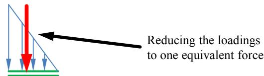
Figure 7. Reducing loadings to one equivalent force if possible
