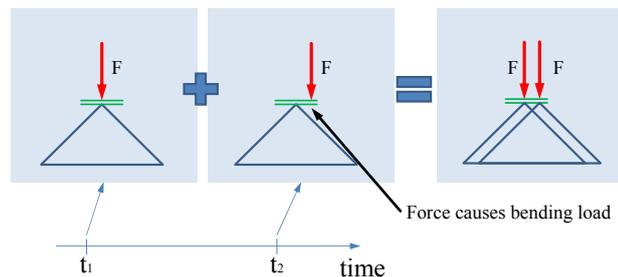
Figure 10. Considering different loadings in different sequences also within one Working Surface Pair
