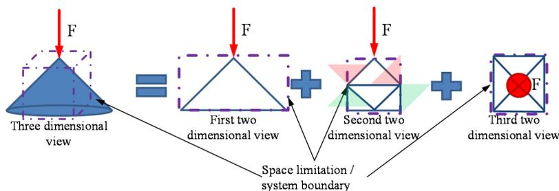
Figure 4. Force Cone and derived structure under consideration of space limitation
