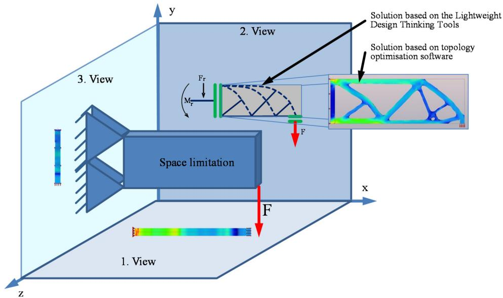
Figure 6. Applying the Lightweight Design Thinking Tools on three dimensional cases
