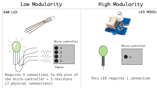
**Figure 1.** Comparing the modularity of two LED components.
