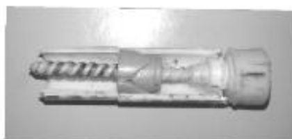
Cross section of mechanism of Fevi Stick Glue
