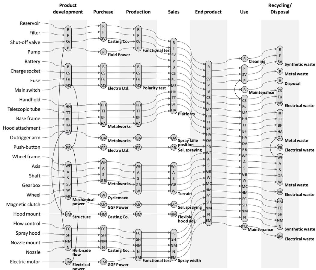
Figure 6. Modularisation of the spraying device over the course of product life
