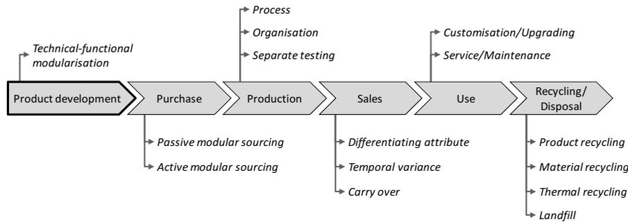
Figure 4. Allocation of the module drivers to the product life phases
