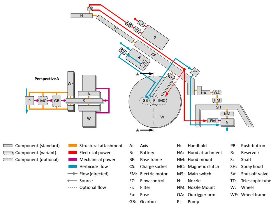
Figure 2. Visualisation of a spraying system by the Module Interface Graph (MIG)
