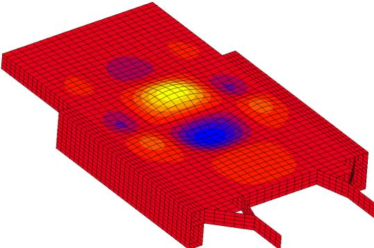
**Figure 4. Buckling of the bottom structure**
