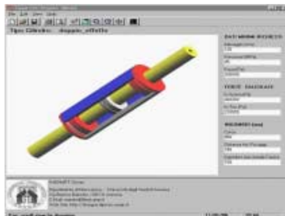
Figure 5. The KBE application user interface with a module instance of the safety brake
