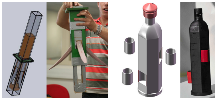
Figure 1. CAD modelisations and prototypes of the anchorage system and the bottle
