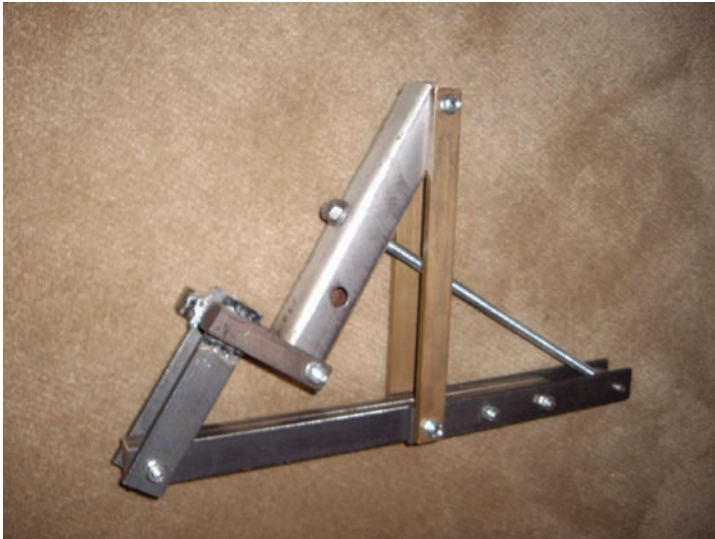
Figure 10. Frame for 2009. The structure is a mechanism until the diagonal power screw is tightened, and students are required to determine the equilibrium configuration.
