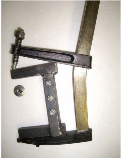
Figure 6. Modified sash cramp with a nut welded onto the screw, and a fabricated 'C' piece with two types of welded joint and a triple-bolted joint in bending. The various notes to students (left) include Vickers Hardness numbers, material, and location of loading position. The failed cramp (right) became unstable before the upper cast iron arm cracked.
