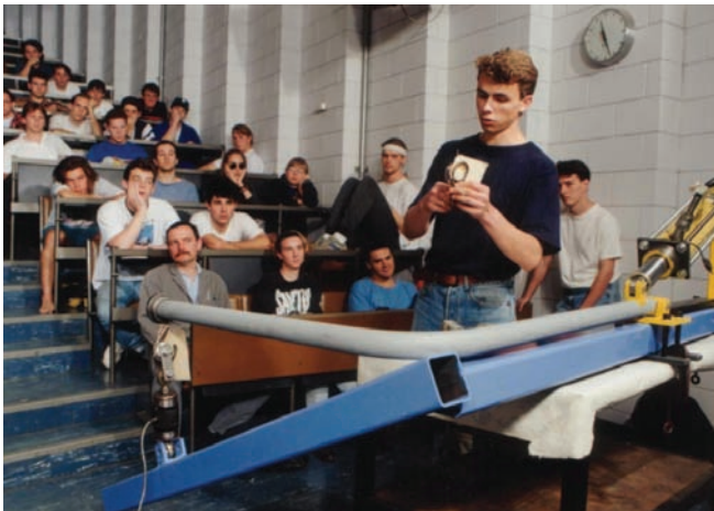
Figure 2. Student-designed crane under destructive test.
