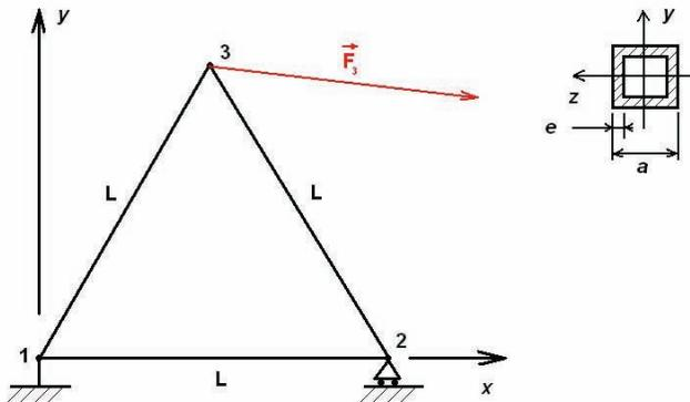
Figure 3 Triangular structure used for the analytical calculation
