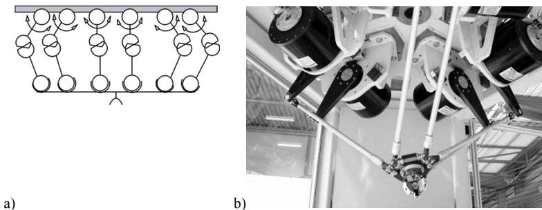
**Figure 3. HEXA robot of the SFB 562: a) kinematic principle, b) photograph**
