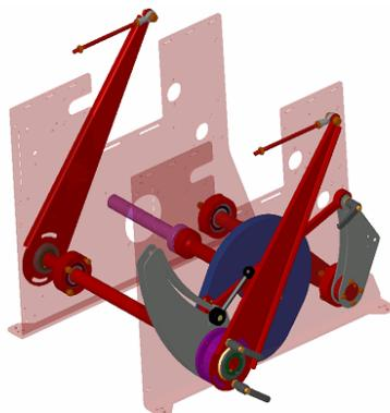
**Figure 2. Original cam unit before optimisation in the constraint modeller**
