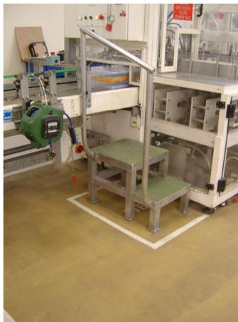
**Figure 1. Typical access steps to a processing machine**
