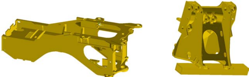
Figure 9. Rear fame (left) and front frame (right) FE models
