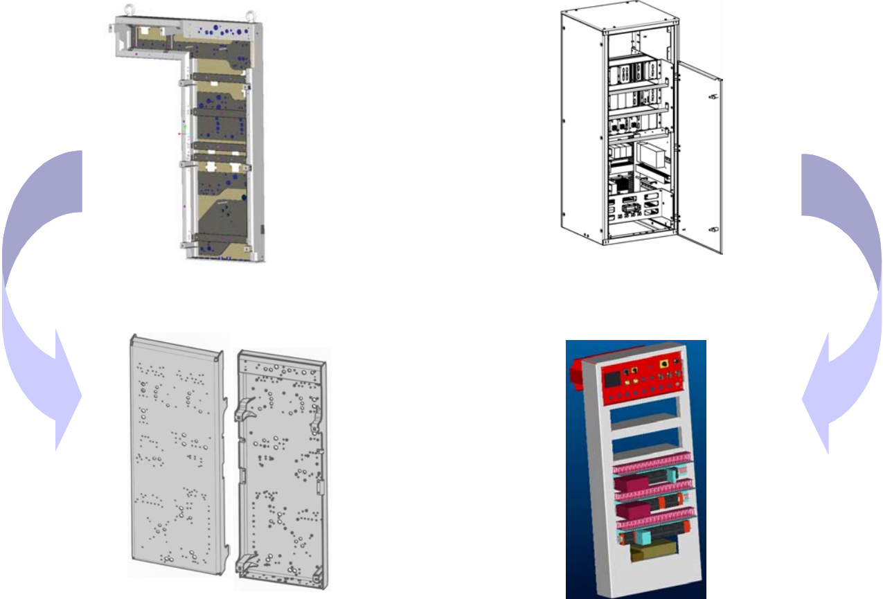
Figure 5: Example of improved modules like the trestle and the control box
