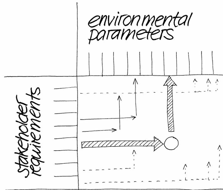
Figure 3. Translating stakeholder requirements into environmental parameter with EQFD [3]
