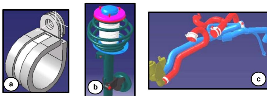
Figure 2. Examples of deformable parts used in A/D context (courtesy BMW): (a) deformable fixing part; (b) spring; (c) flexible hose system.
