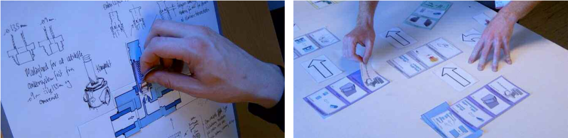
Figure 8. Combining different sub-solutions to visualize alternative product and production concepts. Note that there are added remarks to the concept beside the template of the generic product structure. This could e.g. be remarks on possibilities/constraints linked to the choice of a given sub-solution.
