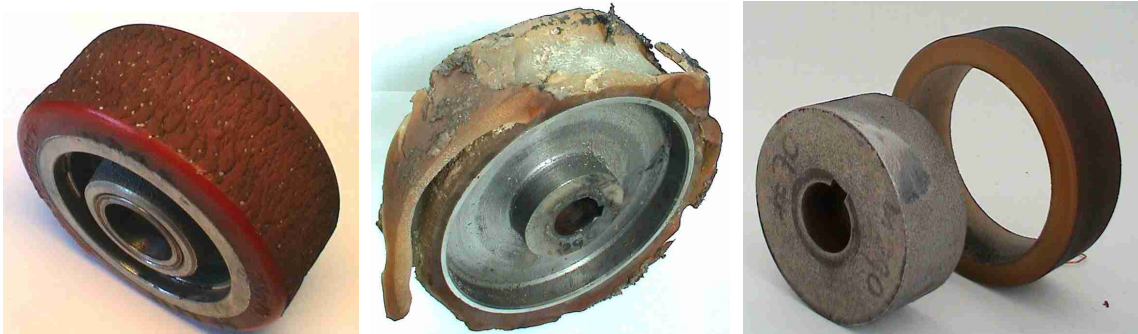
Figure 2. Different failure forms: Abrasive wear, thermal failure, tread delamination
