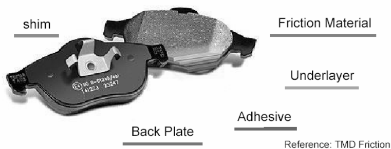
Figure 6. Elements of a Brake pad [www.tmdfriction.com]
