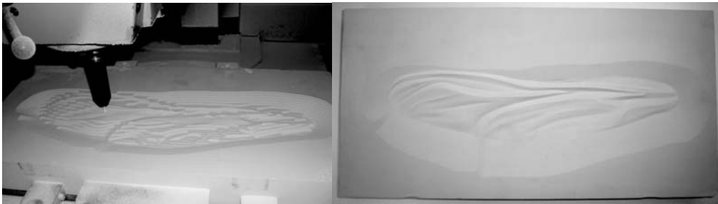
Figure 6. Milling of the cavity and the finished form
